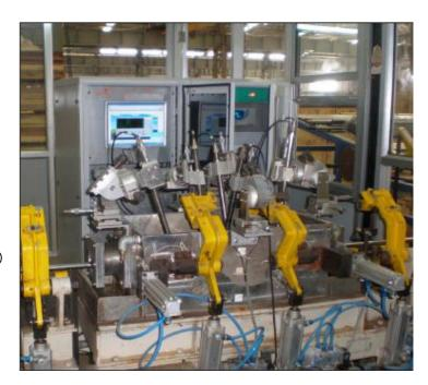
The Seamless Tube test systems is to test the defcets Longitudianally & Transverse oriented defects & Wall thickness measurement including OD/ID based on the International Standard in general E 213, NPCIL or similar, etc. The Test Mechnism will have Immersion tankl having various probes for the defects & wall thickness.
